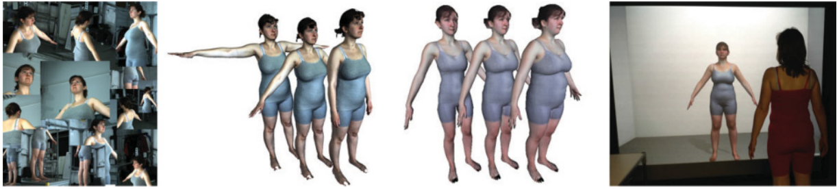
Fig. 1. (From left to right) First, we captured each participant's body geometry and image texture using a 3D scanning system. Second, we captured three poses (T-pose, A-pose, and natural pose), resulting in high-resolution 3D meshes. Third, we fit a statistical model of body shape and pose variation to the scans, bringing them into correspondence; using this model, we created a set of personalized avatars for each subject with varying BMIs (ranging from \pm 20\% BMI change). Fourth, we assessed women's sensitivity to changes in their perceived weight, asking them to estimate whether the size of the participants' personalized avatars displayed on a large-screen immersive display is the same as their current weight.
